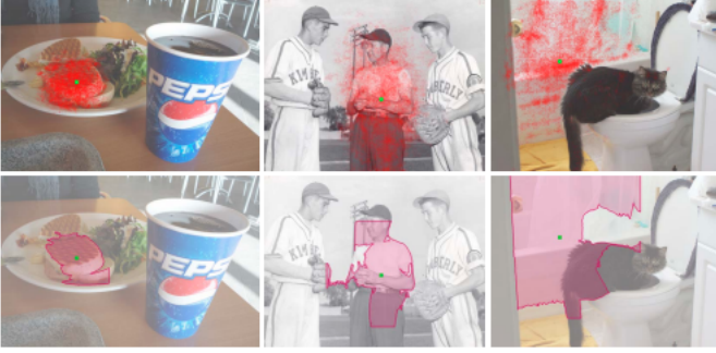
Fig. 2. Example of detected features and resulting segmentation mask using Deformable Convolutions.
